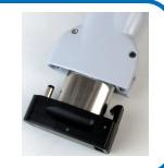
INSERT power key and turn instrument on Note: Yellow light should come on.
