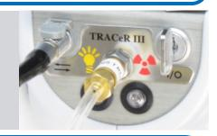
**CONNECT** PDA **or** computer to instrument with serial cable (or USB adaptor if no serial port on computer).
