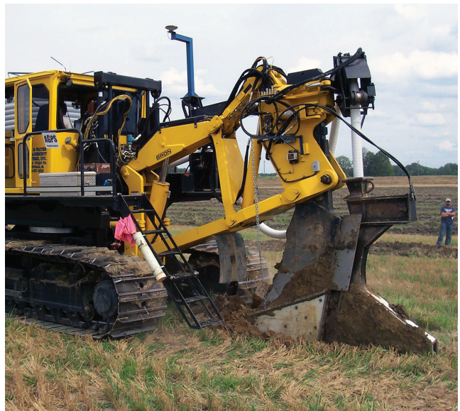
Figure 54 Automatically Guided Trenching Machine
