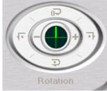
application's control panel • The + and – will rotate the stage in small increments • The outer options will rotate the stage by 90 degrees at a time • If you rotate the specimen, the navigation dials are rotated as well!
