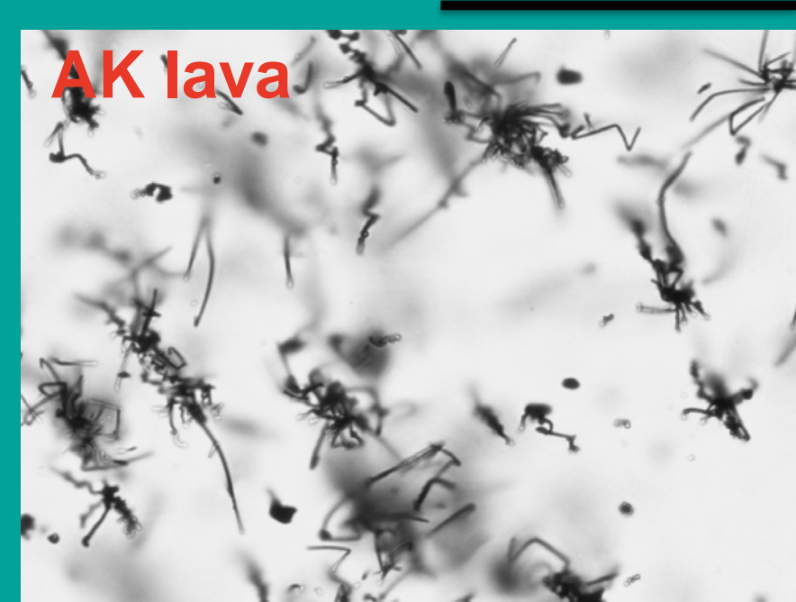
Fig. 3. Photomicrographs showing the oxide morphology in the obsidian from TI and AK lava flows. Scale bar is 100 \mu m.
