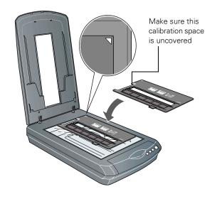
If you are scanning slides, place the holder on the scanner. Then place the slides in the holder. (Place the slides so the "this side to lamp" indication is facing down.)
